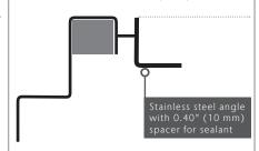
Suitable for heavy duty tiled, paver and resin floor applications, isolates channel from floor and provides gap for sealant. If deeper steel angle required contact ACO.
