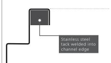
ACO recommends the use of a solid steel edge in-fill when using class E grates or where fork lift traffic is expected.
