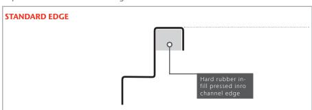
Suitable for tiled, concrete and epoxy resin floors in pedestrian and light industrial applications. Drains without infill are susceptible to failure as the surrounding concrete rarely fills that void. As edges compress, cavities create breeding grounds for pathogens and are impossible to clean. Edge in-fill in other materials - contact ACO for details.
