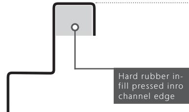
Suitable for tiled, concrete and epoxy resin floors in pedestrian and light industrial applications. Drains without in-fill are susceptible to failure as the surrounding concrete rarely fills that void. As edges compress, cavities create breeding grounds for pathogens and are impossible to clean. Edge in-fill in other materials - contact ACO for details.
