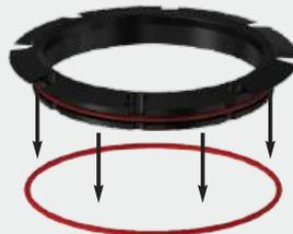
When using adjustable height floor drain with **mechanical membrane clamping flange**, red sealing o-ring must be removed to allow water to enter floor drain body through weep holes on friction ring.
