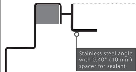
Suitable for heavy duty tiled, paver and resin floor applications, isolates channel from floor and provides gap for sealant. If deeper steel angle required contact ACO.
