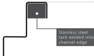
ACO recommends the use of a solid steel edge in-fill when using class E grates or where fork lift traffic is expected.
